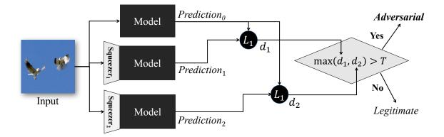
Figure 4.1: Feature-squeezing framework for detecting adversarial examples. The model is evaluated on both the original input and the input after being pre-processed by feature squeezers. If the difference between the model's prediction on a squeezed input and its prediction on the original input exceeds a threshold level, the input is identified to be adversarial.
