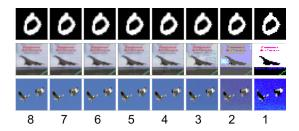
Figure 4.2: Image examples with bit depth reduction. The first column shows images from MNIST, CIFAR-10 and ImageNet, respectively. Other columns show squeezed versions at different color-bit depths, ranging from 8 (original) to 1.
