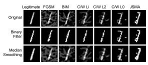
Figure 4.3: Examples of adversarial attacks and feature squeezing methods extracted from the MNIST dataset. The first column shows the original image and its squeezed versions, while the other columns present the adversarial variants. All targeted attacks are targeted-next.
