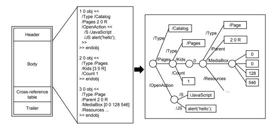
Figure 3.2: The physical and logical structure of a PDF file.
