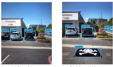
Figure 1.1: An object detection model wrongly recognizes adversarial patch as a car.
