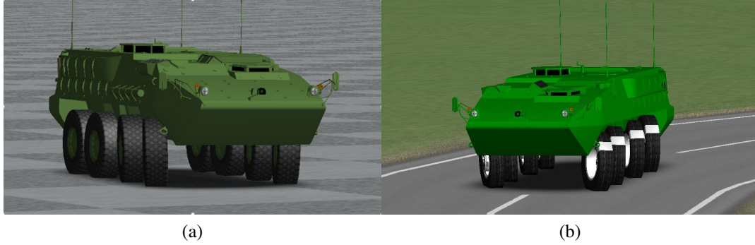
Figure 3.1: Simulated 22 degrees of freedom vehicle model on TruckSim (a) Front-axle steering (b)8-WS vehicle
