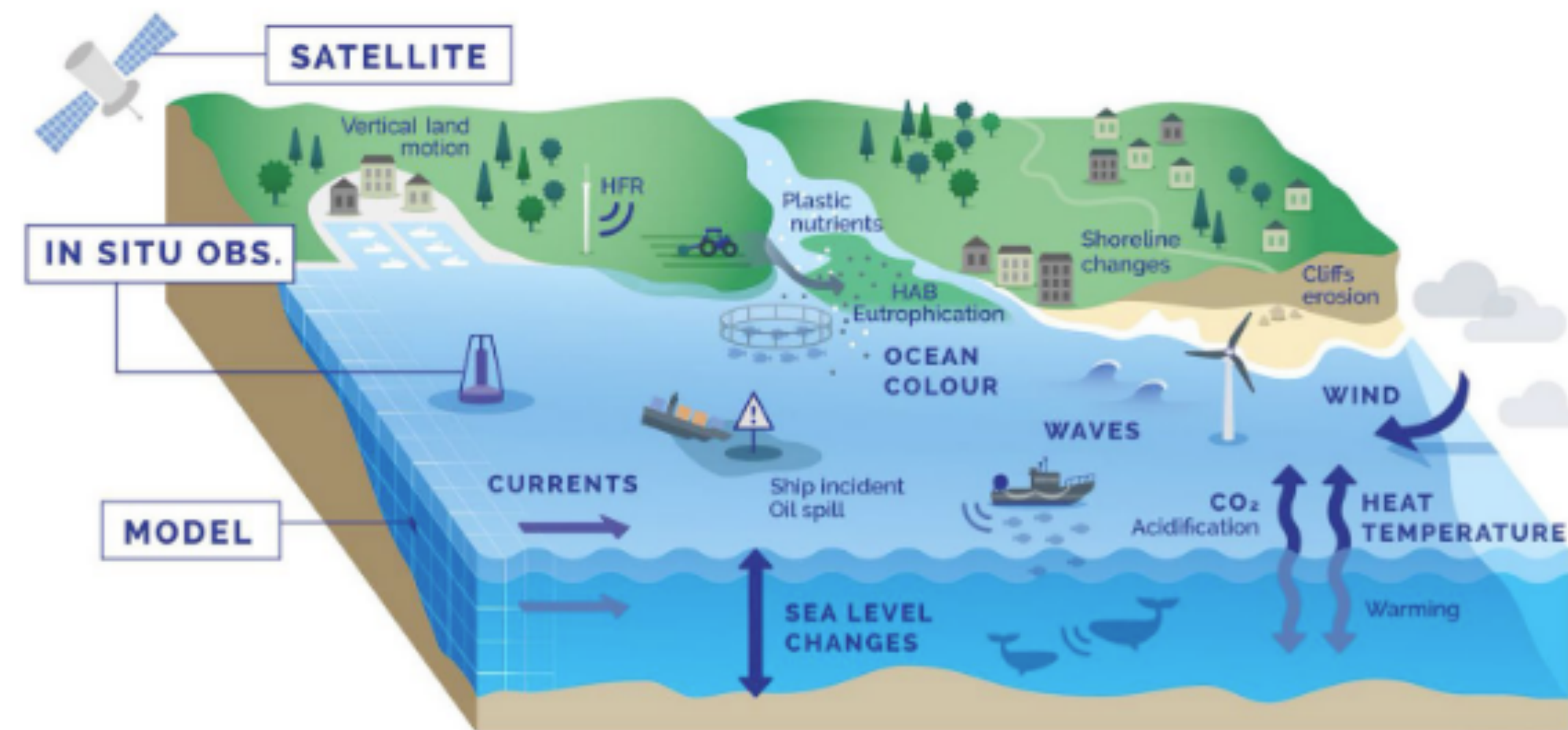
Figure: "Schematic representation of the coastal zone, hazards, and metocean variables that are relevant for coastal marine hazards and their monitoring". Source: [1]
