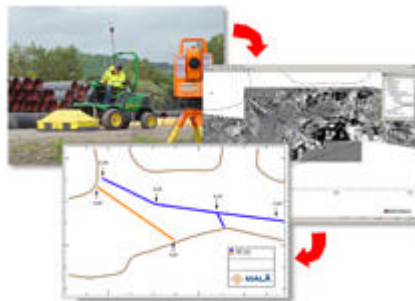
Fig. 1 Detection of the utilities and drafting plans
