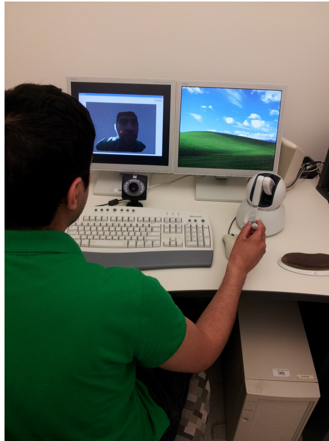
Figure 6.1: A Snapshot of the haptic-enabled Interpersonal Communication System where the user is asked to use the haptic device in addition to mouse and keyboard to communicate with the remote party
