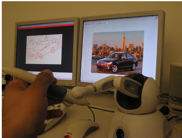
Figure 5.1: A Snapshot of the drawing environment where one monitor's screen shows the required picture to draw and the other screen shows the user's drawing through the haptic device[8]
