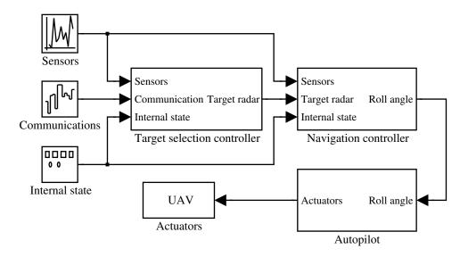
Figure 1: UAV controller architecture
