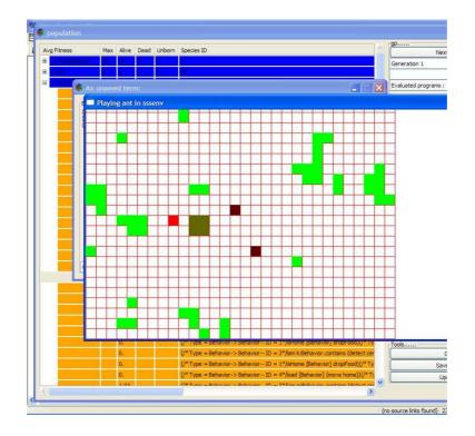
Figure 7.13: The ant cooperation problem interface. The bright red pixel represents an ant carrying food. The other two brown pixels are ants looking for food. The dark green square is the nest and the green patches are the food
