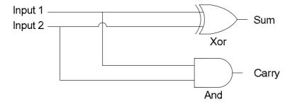
Figure 7.5: A half-adder circuit
