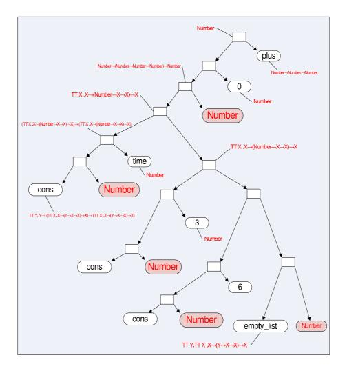
Figure 4.9: A genotype that represents a program that adds all the elements of a list of numbers
