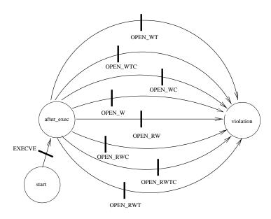
Figure 3.6: State machine for pattern to detect viral behaviour
