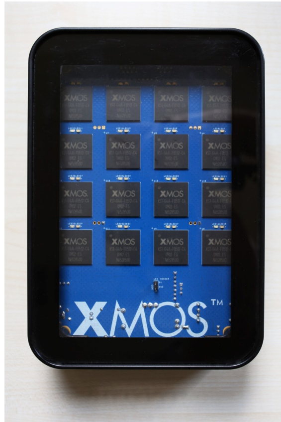
Figure 9.1: The XMOS®XK-XMP-64 platform with an array of 4 \times 4 XS1-G4 quad core CPUs. The size of the housing is 192 mm \times 132 mm \times 46 mm.
