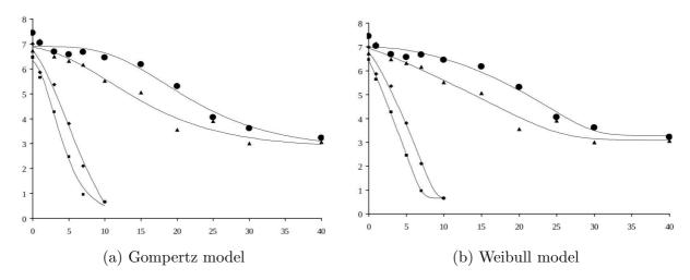
Figure 3.3: Survival curves of Listeria monocytogenes in UHT whole milk during high pressure processing at 350 MPa, 450 MP, 550 MPa, and 600 MPa, generated by the reparameterised Gompertz model, the modified Weibull model
