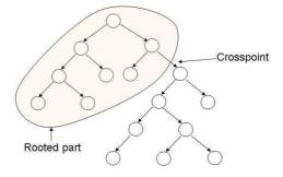
Figure 3.3: The cross-point and the division of the decision tree made by the cut
