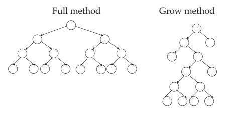
Figure 3.2: The graph representation of the Full and Grow methods to create a new population of programs
