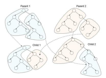
Figure 3.4: A recombination of two parents in order to create a new individual
