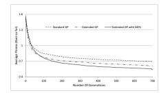
Figure 4. A comparison between "standard GP-Rep". "extended GP-Rep", and "extended GP-Rep with ADFs" on converging to the target melodies. This figure shows an improvement for extended GP-Rep over standard GP-Rep as a result of separating out different dimensions into different branches on the representation tree. Further improvement using ADFs shows up after generation 100. The results are the average of 100 independent runs for each representation (i.e. 10 runs for each target melody).
