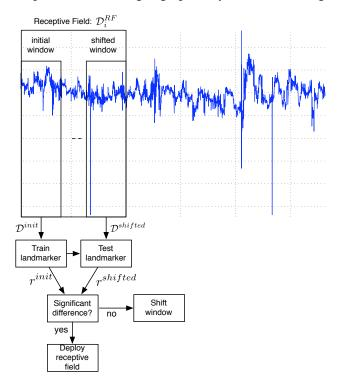
Figure 4.4: A novel receptive field construction process based on concept drift detection
