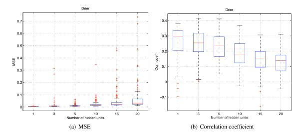
Figure 4.9: Industrial drier: Performance comparison between PCA+MLP-based soft sensors with varying number of hidden units
