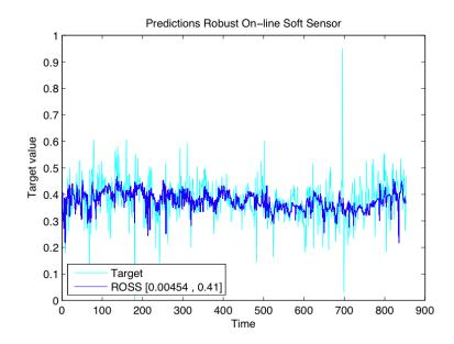
Figure 6.22: Industrial drier: Predictions of the minimal soft sensor (100%) of target values for adaptation)
