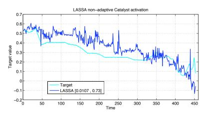
Figure 4.57: Catalyst activation: Predictions of the non-adaptive LASSA-based soft sensor
