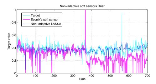
Figure 4.27: Industrial drier: Comparison between a PLS-based soft sensor implemented at Evonik and the non-adaptive version of LASSA-based soft sensor
