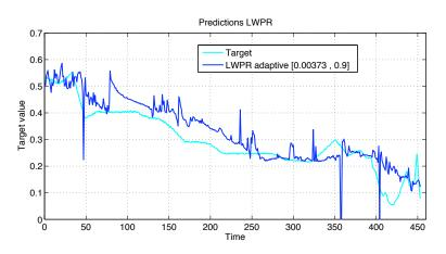
Figure 4.61: Catalyst activation: Predictions of the adaptive LWPR-based soft sensor
