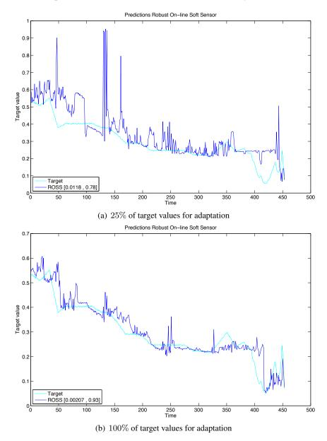
Figure 6.34: Catalyst activation: Predictions of the full-scale soft sensors
