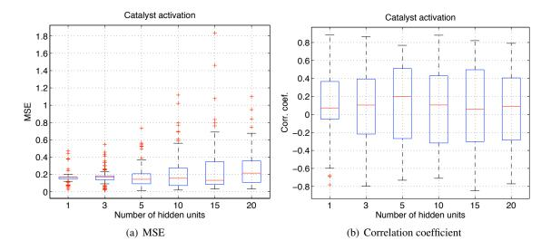
Figure 4.51: Catalyst activation: Performance comparison between combined PCA+MLP-based soft sensors with varying number of hidden units
