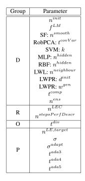
Table 6.3: Input parameters of the complex soft sensing algorithm and their allocation to the different parameter classes
