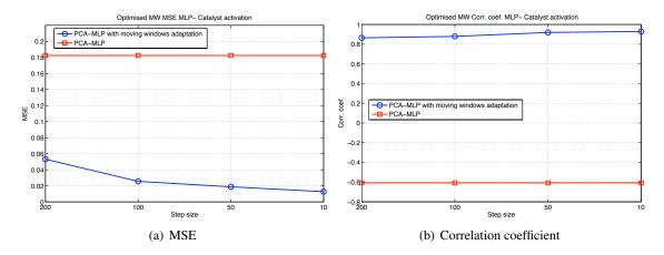
Figure 4.58: Catalyst activation: Effect of the moving window step size on the performance of the adaptive PCA+MLP-based soft sensor
