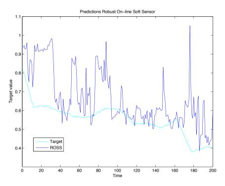
Figure 6.41: Catalyst activation: Minimal training data soft sensor predictions (detail view of the first 200 samples)
