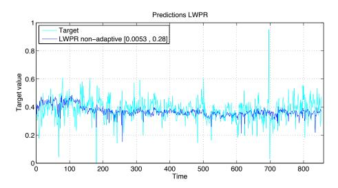
Figure 4.15: Industrial drier: Predictions of the non-adaptive LWPR-based soft sensor
