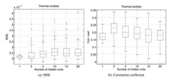
Figure 4.33: Thermal oxidiser: Performance comparison between combined PCA+MLP-based soft sensors with varying number of hidden units
