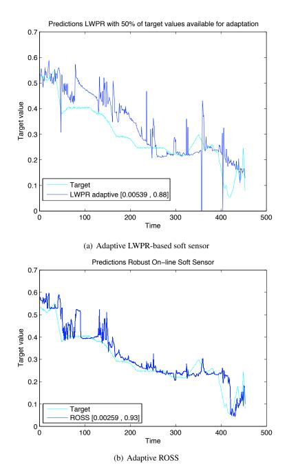
Figure 6.20: Catalyst activation: Predictions of two adaptive soft sensors using 50% of target values for adaptation
