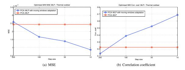
Figure 4.41: Thermal oxidiser: Effect of the moving window step size on the performance of the adaptive PCA+MLP-based soft sensor
