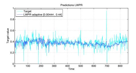
Figure 4.22: Industrial drier: Predictions of the adaptive LWPR-based soft sensor
