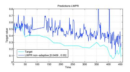
Figure 4.54: Catalyst activation: Predictions of the non-adaptive LWPR-based soft sensor
