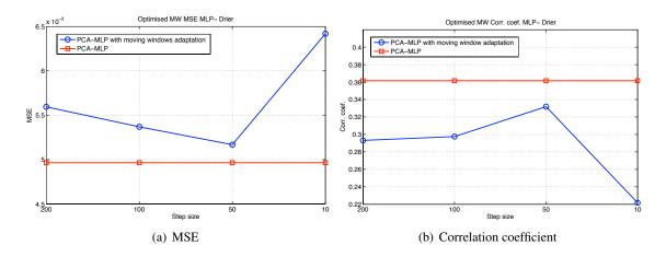
Figure 4.20: Industrial drier: Effect of the moving window step size on the performance of the adaptive PCA+MLP-based soft sensor
