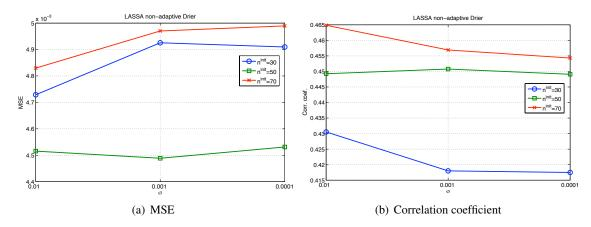
Figure 4.16: Industrial drier: Influence of  $n^{init}$  and  $\sigma$  on the performance of the non-adaptive LASSA-based soft sensor
