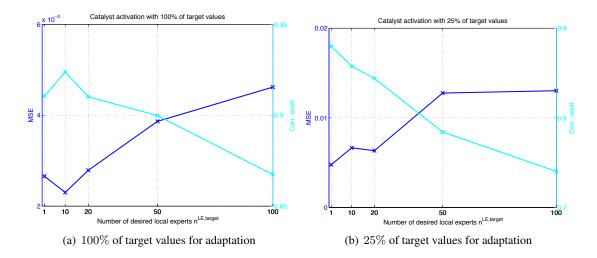
Figure 6.14: Catalyst activation: The MSE and correlation coefficients achieved with different population sizes
