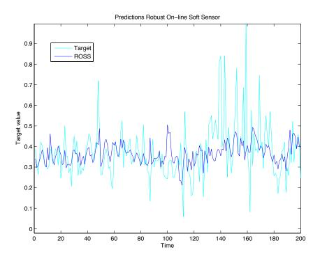
Figure 6.37: Industrial drier: Minimal training data soft sensor predictions (detail view of the first 200 samples)
