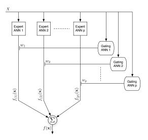
Figure 3.3: Gating Artificial Neural Network structure
