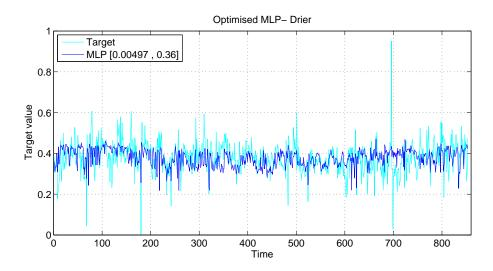
Figure 4.13: Industrial drier: Predictions of the non-adaptive PCA+MLP-based soft sensor
