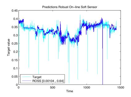
Figure 6.26: Thermal oxidiser: Predictions of the minimal soft sensor (100% of target values for adaptation)
