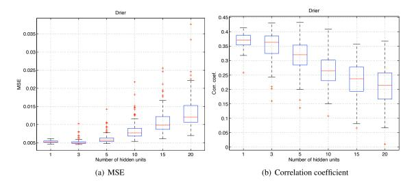
Figure 4.11: Industrial drier: Performance comparison between combined PCA+MLP-based soft sensors with varying number of hidden units
