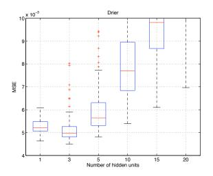
Figure 4.12: Industrial drier: MSE performance comparison between combined PCA+MLP-based soft sensors with varying number of hidden units - detailed view
