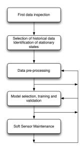
Figure 2.4: A soft sensor development methodology
