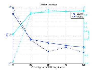
Figure 6.18: Catalyst activation: The effects of changing amount of target values, comparison between the LWPR-based soft sensor and ROSS (note the logarithmic left-hand side y-scale)
