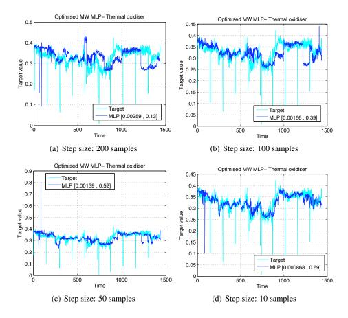
Figure 4.42: Thermal oxidiser: Effect of the adaptation of the PCA+MLP soft sensor using the moving window technique
