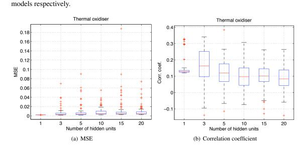
Figure 4.31: Thermal oxidiser: Performance comparison between PCA+MLP-based soft sensors with varying number of hidden units
