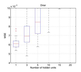
Figure 4.10: Industrial drier: Performance comparison between PCA+MLP-based soft sensors with varying number of hidden units - detailed view
