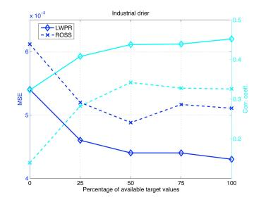
Figure 6.15: Industrial drier: The effects of changing amount of target values, comparison between the LWPR-based soft sensor and ROSS
