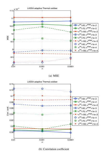
Figure 4.45: Thermal oxidiser: Influence of  $n^{init}$ ,  $\sigma$  and  $\sigma^{adapt}$  on the performance of the adaptive LASSA-based soft sensor
