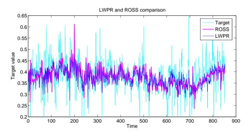
Figure 6.32: Industrial drier: Direct comparison between the LWPR-based soft sensor and ROSS
