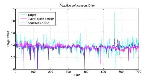
Figure 4.28: Industrial drier: Comparison between the adaptive PLS-based soft sensor implemented at Evonik and the adaptive LASSA-based soft sensor.
