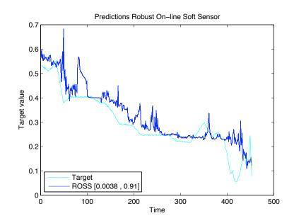
Figure 6.28: Catalyst activation: Predictions of the minimal soft sensor (100% of target values for adaptation)
