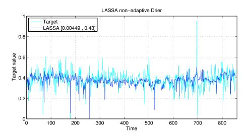
Figure 4.19: Industrial drier: Predictions of the non-adaptive LASSA-based soft sensor
