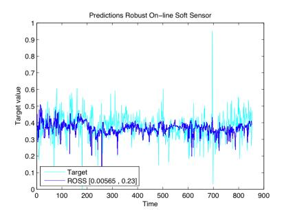
Figure 6.24: Industrial drier: Predictions of the minimal soft sensor (25%) of target values for adaptation)
