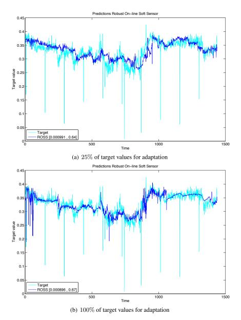
Figure 6.33: Thermal oxidiser: Predictions of the full-scale soft sensors
