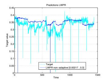
Figure 4.36: Thermal oxidiser: Predictions of the non-adaptive LWPR-based soft sensor
