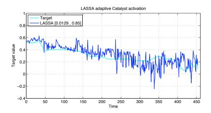
Figure 4.63: Catalyst activation: Predictions of the adaptive LASSA-based soft sensor
