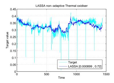
Figure 4.39: Thermal oxidiser: Predictions of the non-adaptive LASSA-based soft sensor
