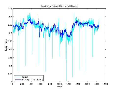
Figure 6.38: Thermal oxidiser: Predictions of a soft sensor developed using minimal training data
