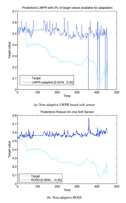
Figure 6.19: Catalyst activation: Low performance of the non-adaptive soft sensors
