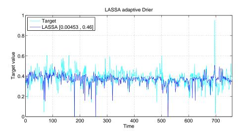
Figure 4.26: Industrial drier: Predictions of the adaptive LASSA-based soft sensor
