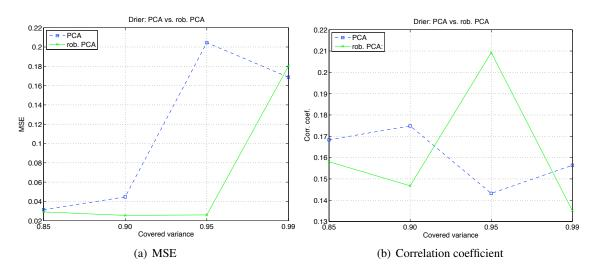
Figure 4.7: Industrial drier: Comparison between the performances achieved with PCA and robust PCA pre-processing for varying settings of variance contained in the principle components, i.e. varying numbers of resulting principle components
