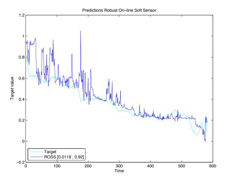
Figure 6.40: Catalyst activation: Predictions of a soft sensor developed using minimal training data
