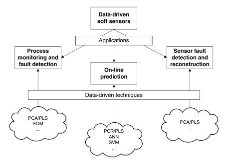
Figure 1.2: Overview of application areas of data-driven soft sensors
