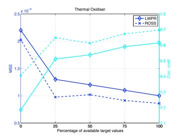
Figure 6.16: Thermal oxidiser: The effects of changing amount of target values, comparison between the LWPR-based soft sensor and ROSS
