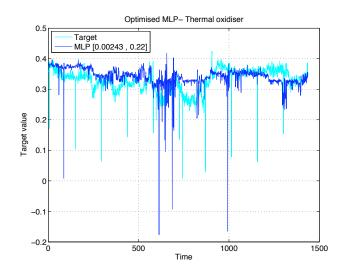
Figure 4.34: Thermal oxidiser: Predictions of the non-adaptive PCA+MLP-based soft sensor
