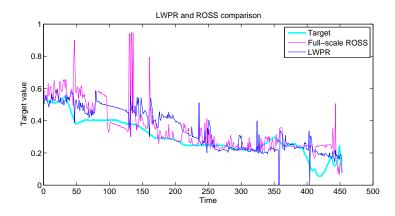
Figure 6.35: Catalyst activation: Direct comparison between the LWPR-based soft sensor and ROSS (25% of target data for adaptation)
