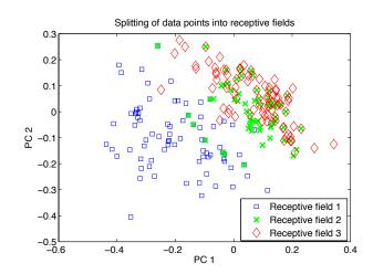
Figure 6.2: Splitting of data points into three receptive fields (displayed after projection to twodimensional space by means of principal component analysis)
