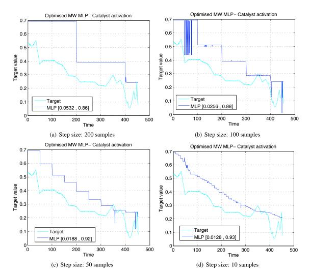
Figure 4.59: Catalyst activation: Effect of the adaptation of the PCA+MLP soft sensor using the moving window technique
