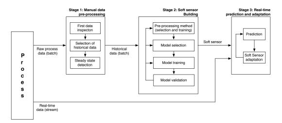
Figure 4.3: Detailed overview of the proposed soft sensor development and maintenance methodology
