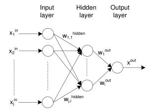
Figure 3.2: Multi-Layer Perceptron structure (without bias connections)
