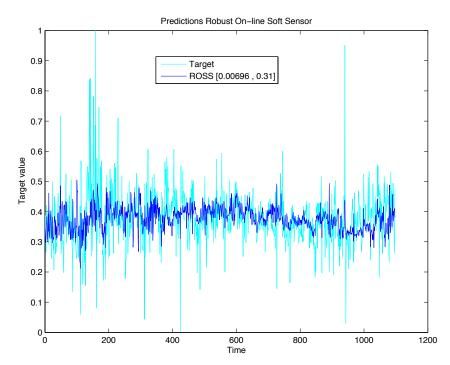
Figure 6.36: Industrial drier: Predictions of a soft sensor developed using minimal training data
