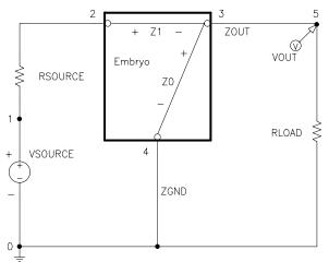
Figure 1 One-input, one-output initial circuit.
