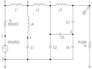
Figure 2 Genetically evolved parameterized filter.
