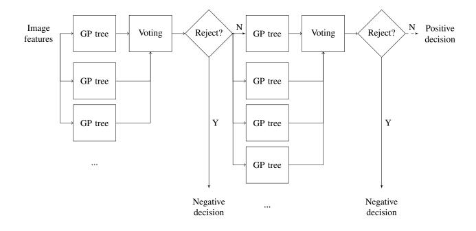
Fig. 2. The cascade of voting committees of GP classifiers. Each cascade node is a set of GP trees that make independent decisions that are subsequently aggregated via voting. In both training and testing, only the examples classified as positive by a cascade node reach the subsequent node. An example has to pass through all cascade nodes to become ultimately classified as positive.
