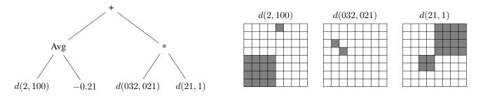
Fig. 3. An exemplary GP tree (left) and the image features fetched by its terminal nodes (right). Each feature is a difference of total brightness in two rectangular regions addressed by quad-tree codes. For clarity, only three uppermost levels are illustrated by the grid, so that it corresponds to the entire  $32 \times 32$  input window and a single grid cell corresponds to a square of  $4 \times 4$  pixels.
