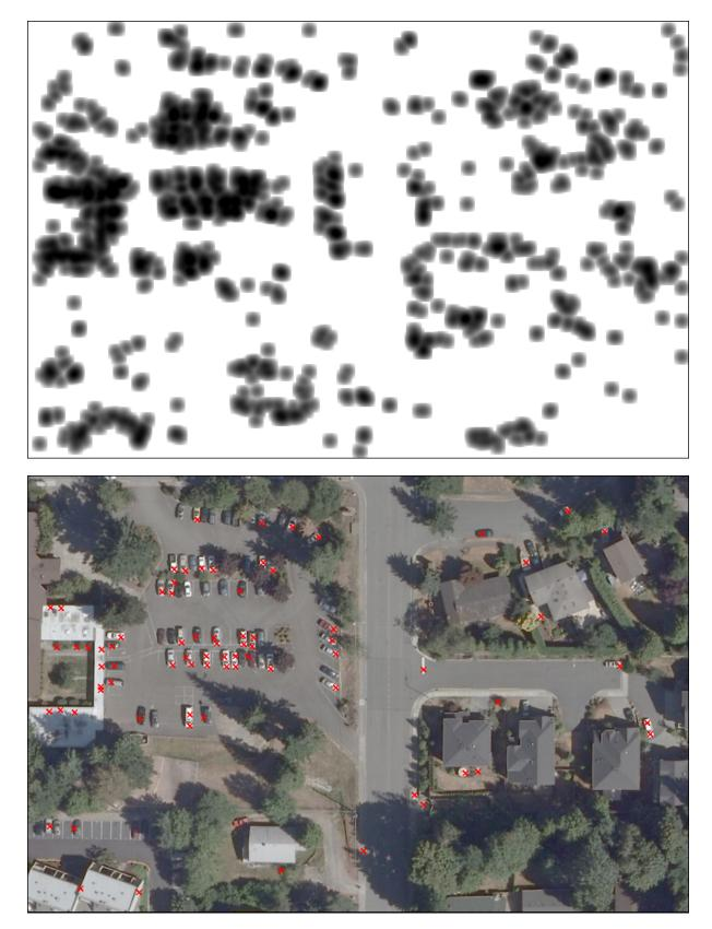
Fig. 5. Detection density map DDM (top) and the corresponding final detection result (bottom). For the DDM, the darker the pixel, the more evidence has been collected for the presence of vehicle at a particular location. In the bottom image, red crosses indicate the positive decisions of the system.
