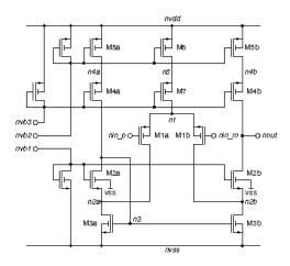
Figure 2. Schematic of high-speed CMOS OTA
