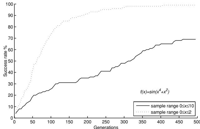
**Figure 6.** The relationship between success rate and generations for the test problem  $T_2$  using the RRGP representation. Two sample ranges for the test cases are shown. Compare these ranges with Figure 5. The solid black line is most comparable with the results shown in Figure 1.
