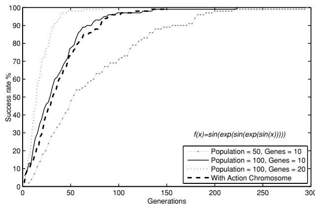
**Figure 7.** The relationship between success rate and generations for the test problem  $T_3$  using the RRGP representation. Four variations of the configuration are shown. Notice that where the action chromosome is included the population is 100 and the individuals have 20 genes, this is shown with the thick dashed line. The plot shown with the dotted line, representing a population of 100 and 20 genes is most comparable to the plot in Figure 1.
