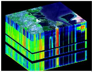
Figure 1:Hyper-spectral image cube of AVIRIS data from NASA.
