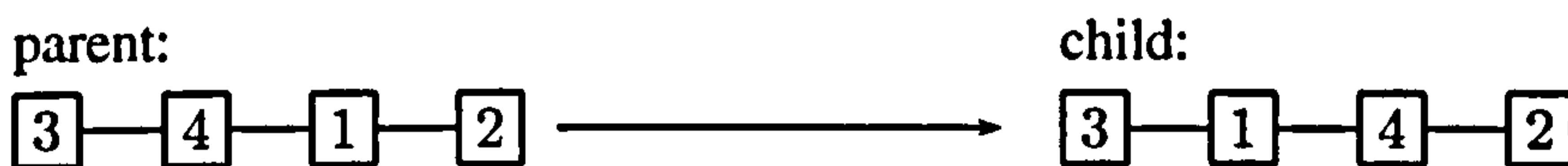
Fig. 62: Example of the second type of crossover.
