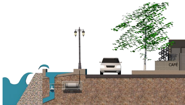
Figure 4: Sketch of the Overtopping Device WEC Concept
