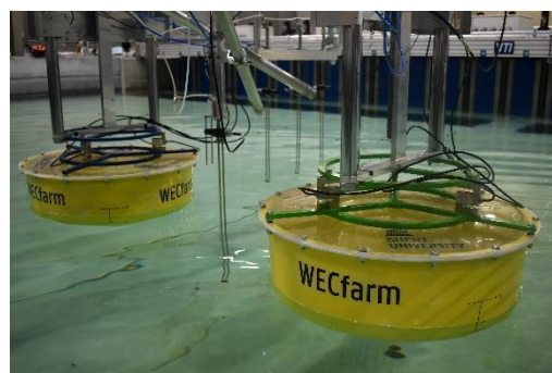
Figure 1: Experimental setup with the WECfarm two-WEC array at the AAU wave basin.
