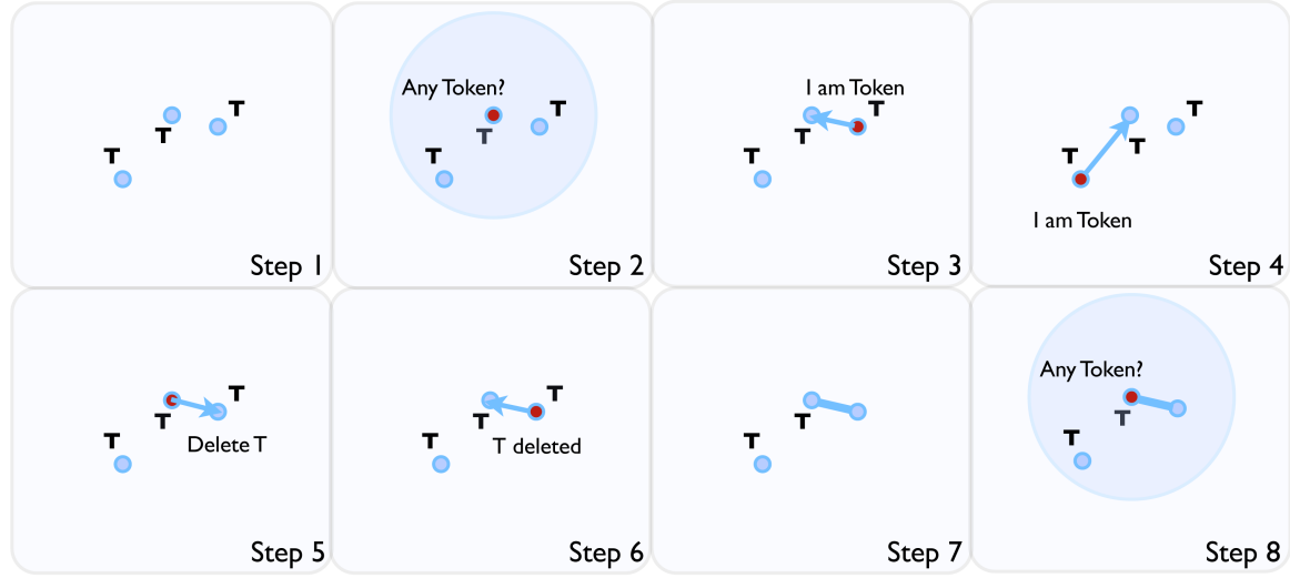
Figure 6.3: Steps in the creation of a tree topology in the network.
