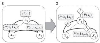
**Fig. 3.** (a) Bayesian network and (b) Factor graph. Dotted lines represent tree structures. Circles are variable nodes and lozenges are factor nodes. (b) is equivalent to (a).
