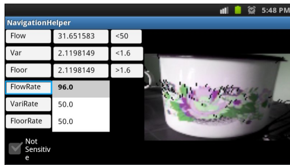
Figure12: Confidence of agents when the camera is pointed towards a colorful obstacle.
