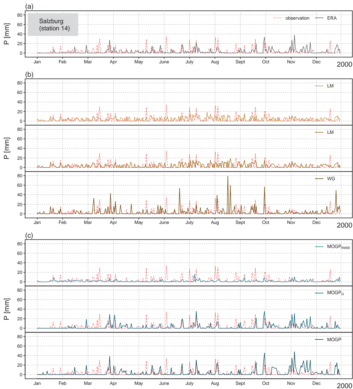
Figure 7.13.: Time series of daily accumulated precipitation P as observed, from ERA-Interim and from the different downscaling techniques at Salzburg (station 14) in the year 2000. The dashed red lines show the observations. The solid lines show the precipitation from ERA-Interim and from the different downscaling approaches.
