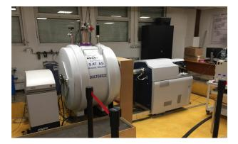
Figure 3.1: FT-ICR device (photo taken at the MSAP laboratory, University of Lille)
