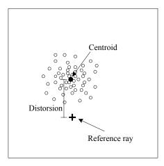
Figure 4: Illustration of the Blur Spot Measure
