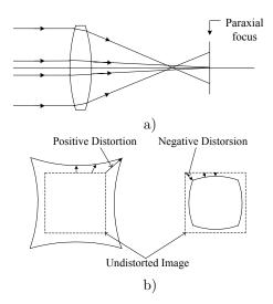
Figure 3: Illustration of: a) Spherical Aberration, and b) Distortion.
