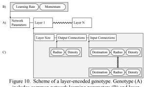
includes common network learning parameters (B) and layer parameters (C).
