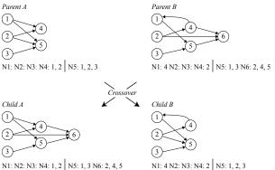
Figure 4. Example of node-based network encoding. Vertical lines in genotype transcription represent crossover points.
