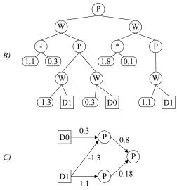
Figure 5. Example of node-based encoding by the means of genetic programming. LISP expression (A) is used as a tree (B) from which the network is constructed (C).
