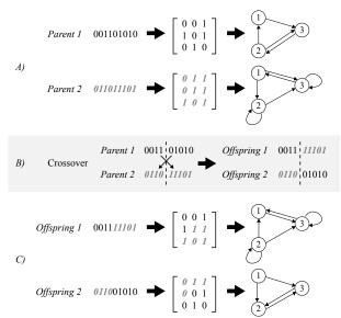
Figure 3. Application of crossover operator on connection matrix encoded network. Parent bit string chromosomes (A) are crossed over at random position (B) to create offspring (C) like in classical genetic algorithm.
