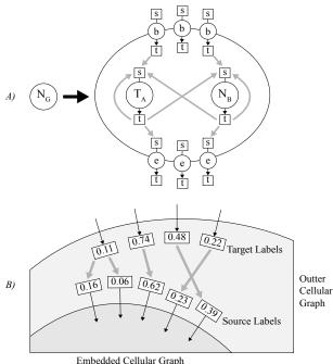
Figure 14. Basic elements of a cellular graph grammar encoding. (A) displays a general rewrite rule with non-terminal on the left side and a cellular graph on the right side with possible connections for source and target labels. When  $N_B$  in the rewrite rule is replaced by another cellular graph, the embedded cellular graph is connected to the outer by similar source and target labes (B).
