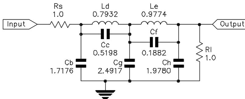
Figure 3: Equally-terminated elliptic filter
