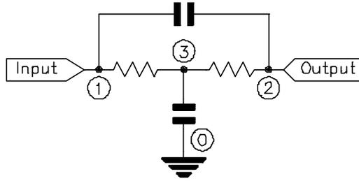
Figure 1: Bridged-T filter
