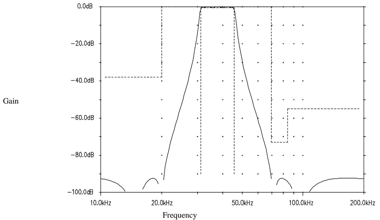
**Figure 9: Frequency response of 10th-order elliptic band-pass filter**
