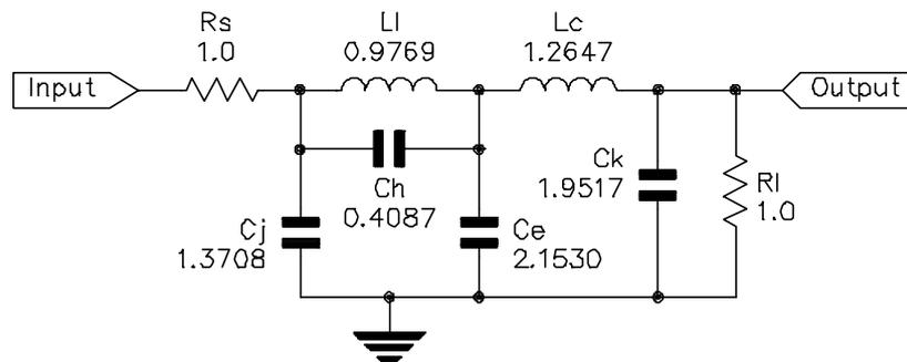
**Figure 7: Hybrid-GA designed equally-terminated filter**
