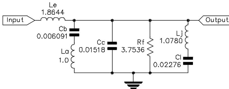
**Figure 12: Hybrid-GA designed averaging filter**
