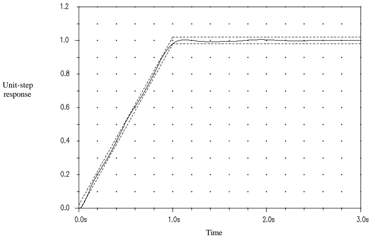
**Figure 13: Unit-step response of hybrid-GA designed averaging filter**
