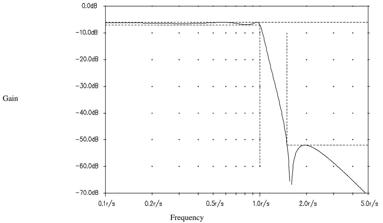
**Figure 8: Frequency response of hybrid-GA designed equally-terminated filter**
