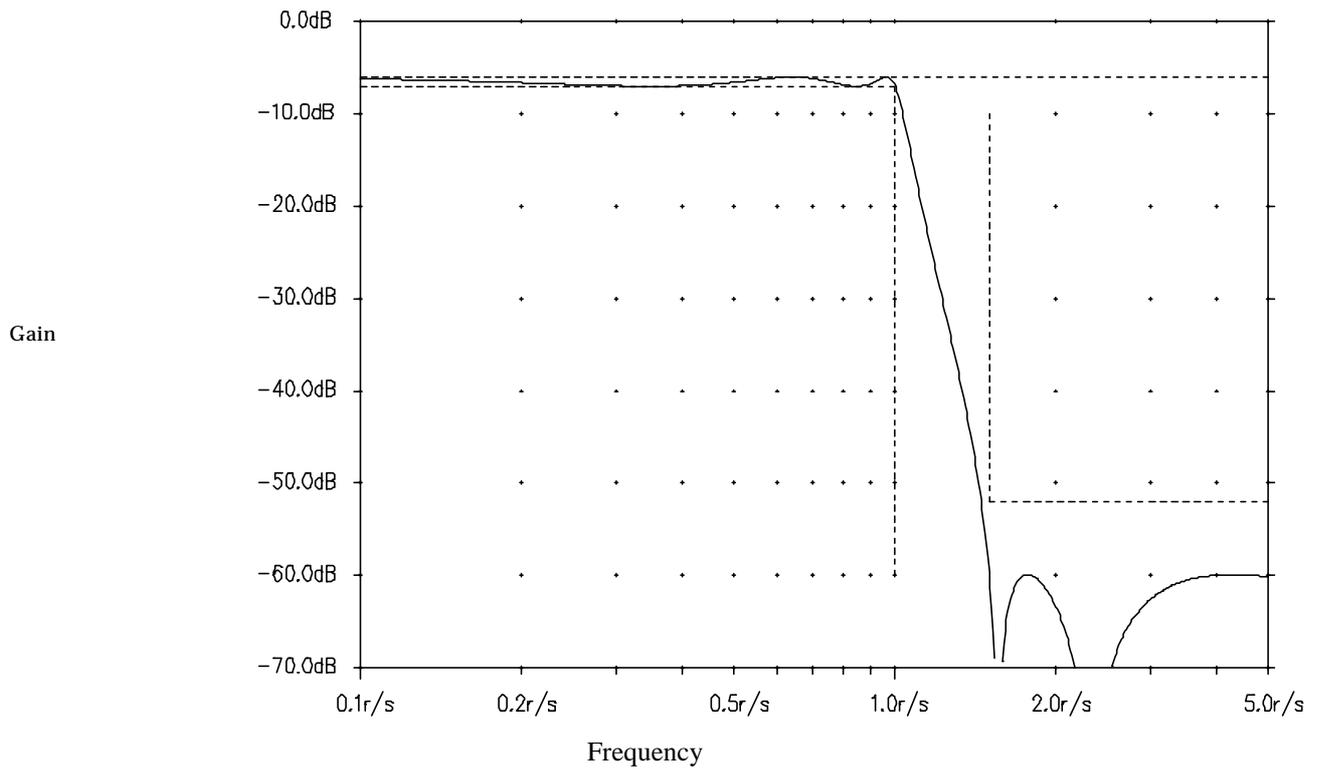
**Figure 4: Frequency Response of elliptic filter**
