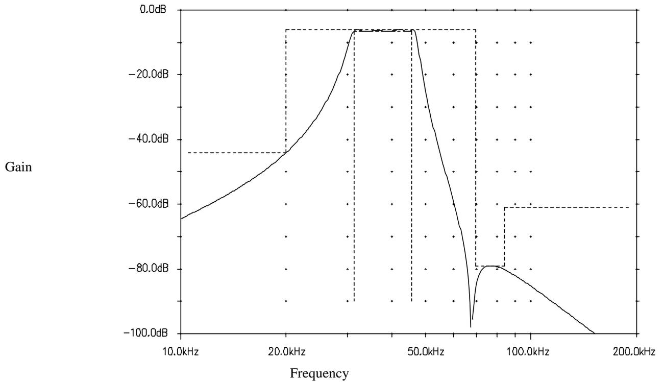
**Figure 11: Frequency response of hybrid-GA designed Nielsen filter**
