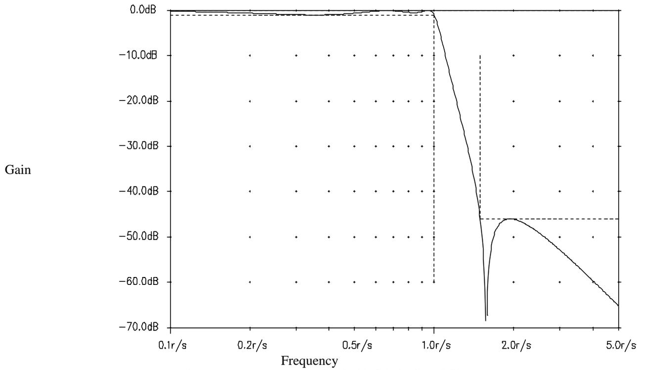
**Figure 6: Frequency response of hybrid-GA designed filter**
