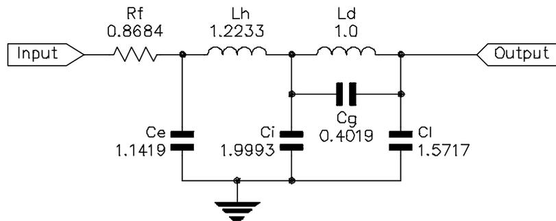
**Figure 5: Hybrid-GA designed filter**
