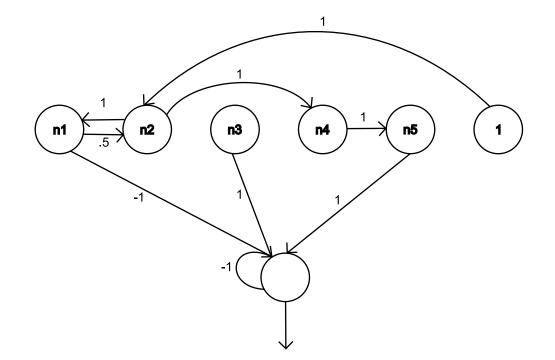
Figure 2: Solution to 5-parity
