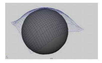
Figure 4: This surface is pulled downwards by gravity, but it is blocked by the sphere.
