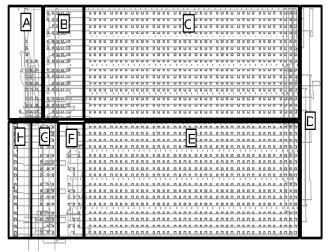
Figure 2 Arrangement of elements A through H on a  $32 \infty 64$  portion of the XC6216 chip.
