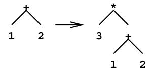
Figure 1: Example of the macro mutation operator insert\_internal. The '+' node is chosen for mutation, and is moved to a new location. A new node '\*' is inserted in the old position and one of its two branch points is connected back to the '+'. The remaining branch point for the '\*' function is filled out with a new tree, which in this case is just a single node '3'.
