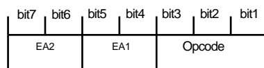
Figure 4. Layout of an instruction where there are eight possible opcodes and two effective addresses. The details of what the opcodes do and the effective addresses is problem specific.
