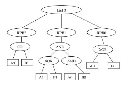
Figure 1: Illustration of First Approach on a 2-bit Adder
