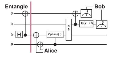
Figure 7. With one bit of prior entanglement we can communicate two c-bits through  $BS(\pi)$  without error (discovered by genetic programming).
