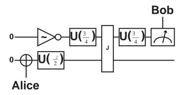
Figure 5. The strategy discovered for the Smolin gate works for any instance of  $J(\theta)$  with zero error.
