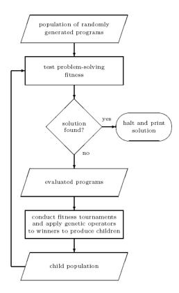
Figure 8. Flowchart of the genetic programming algorithm.
