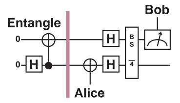
Figure 6. With one bit of prior entanglement we can communicate one c-bit through  $BS(\frac{\pi}{4})$  without error (discovered by genetic programming).
