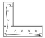
Fig. 2. The motion of one of the best robots found by the EA. The squares in the upper right, lower left, and lower right corners represent the charging stations.
