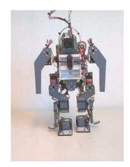
Fig. 1. Picture of the humanoid robot 'elvina'.
