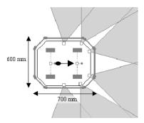
Figure 2: The upper view of CAT. The sonar sensibility cones are represented in gray, and the bumpers as solid lines around the robot body.
