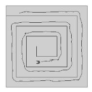
Figure 4: The environment for the experiments with Q-learning and Bucket Brigade, and one of the learnt fuzzy behaviors: CAT (black and white dot) starts from the center and goes along the corridors.
