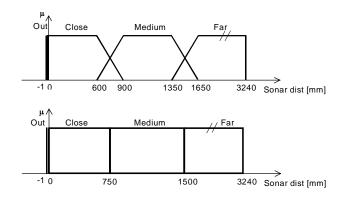
Figure 1: The fuzzy membership functions (above) and the intervals (below) to interpret the distance measured by a sonar sensor, used in the antecedents of, respectively, fuzzy and crisp classifiers presented in Section 4.
