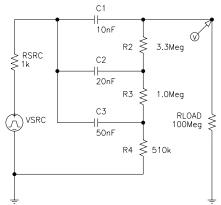
Figure 1 Philbrick 1956 circuit consisting of three capacitors and three resistors.
