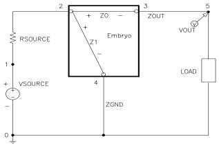
Figure 3 One-input, one-output initial circuit with two modifiable wires, source resistor, and variable load.
