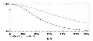
Figure 11 Comparison of time-domain behaviors of the 1956 Philbrick circuit (top curve without boxes) and the best circuit from generation 39 (bottom curve with boxes).
