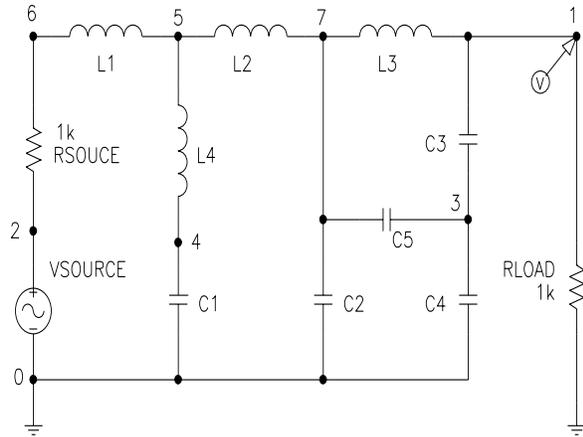
**Figure 2 Genetically evolved parameterized filter.**
