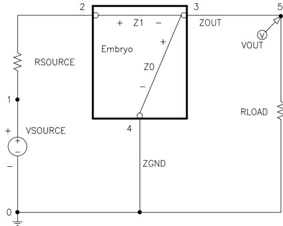
Figure 1 One-input, one-output initial circuit.
