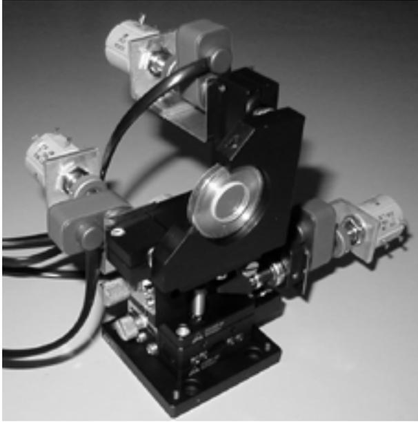
Figure 3: Photograph of the Mirror Holder Incorporated with Three Picomotors and Potentiometers
