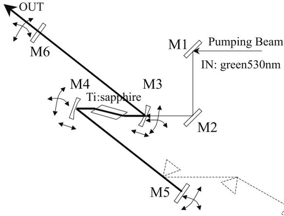
Figure 4: Cavity Configuration for the Ti:sapphire Laser
