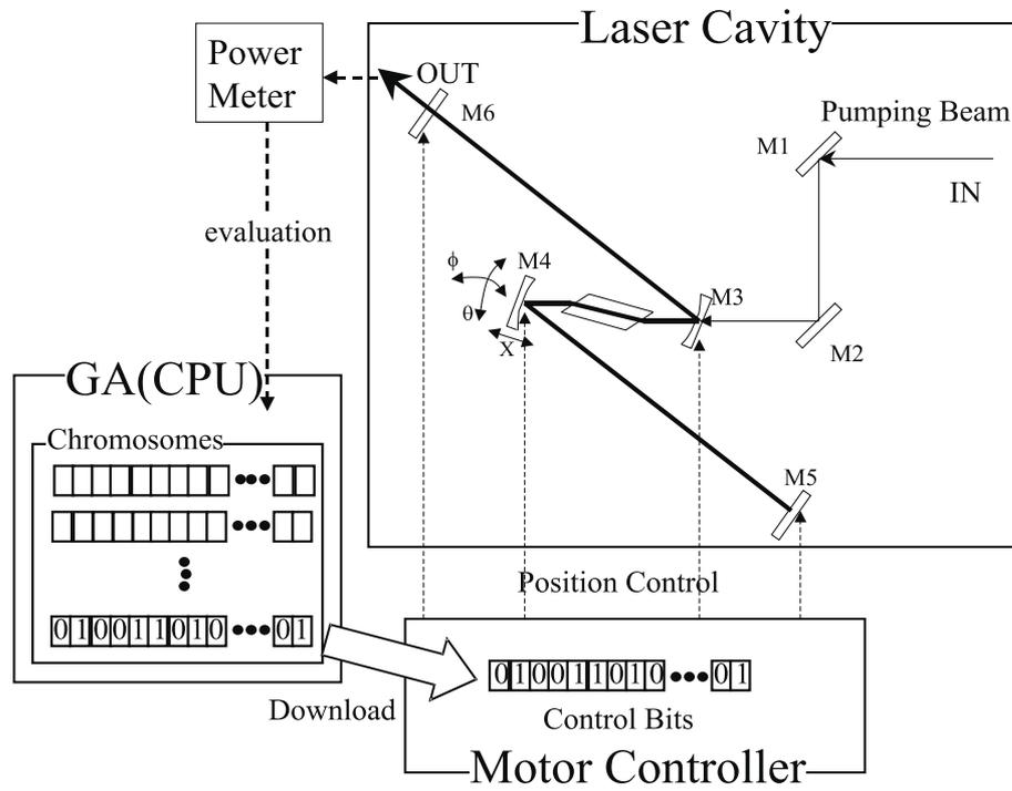
Figure 1: Schematic Representation of the Evolvable Laser System
