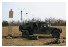
Figure 2: HMMVV with two Boomerang sensors mounted on back
