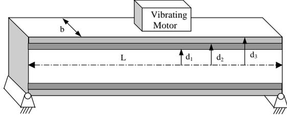
Figure 4: Vibrating platform design problem.
