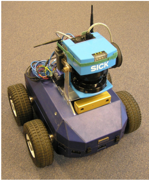
Figure 8: The robotic vehicle (an Applied AI GAIA) used for real-world training, with its SICK LMS-200 laser rangefinder and Point Grey Bumblebee digital stereo camera.
