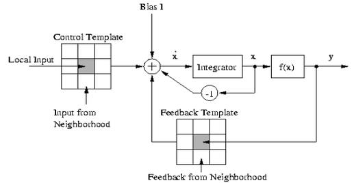
Fig.2 CNN System block diagram of a cell  $C(i,j)$
