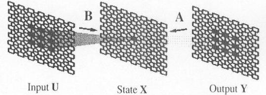
Fig.1 Signal flow structure of a CNN
