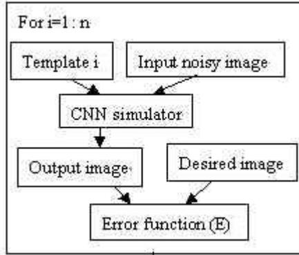
Fig.5: The flow chart of CNN simulator.
