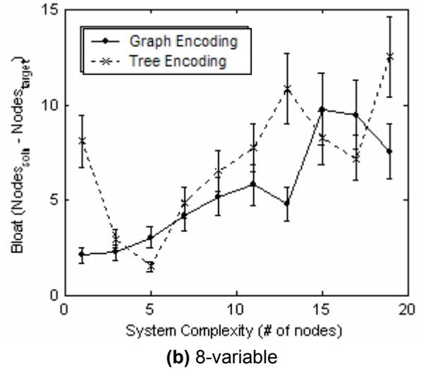
**Figure 2. Bloat of converged solutions for 1-variable functions (a), and 8-variable functions (b). Each point is averaged over 50 randomly generated target functions. Error bars show the standard error.**
