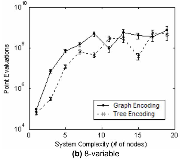
**Figure 4.** The number of point evaluations before convergence on the training set versus the target function complexity for 1-variable functions (a), and 8-variable functions (b). Each point is averaged over 50 randomly generated target functions. Error bars show the standard error.
