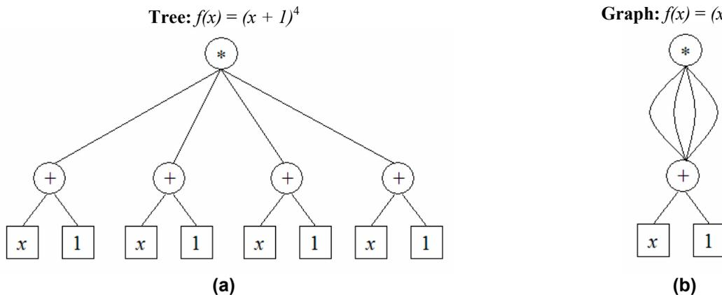
**Figure 1.** Example expressions of  $f(x) = (x + 1)^4$  in the tree encoding (a) and graph encoding (b). The graph encoding reuses redundant sub-expressions but is more susceptible to deleterious variation.
