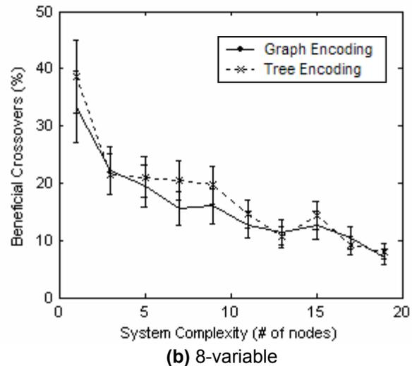
**Figure 5.** The rate of beneficial crossovers versus target function complexity for 1-variable functions (a), and 8-variable functions (b). Each point is averaged over 50 randomly generated target functions. Error bars show the standard error.
