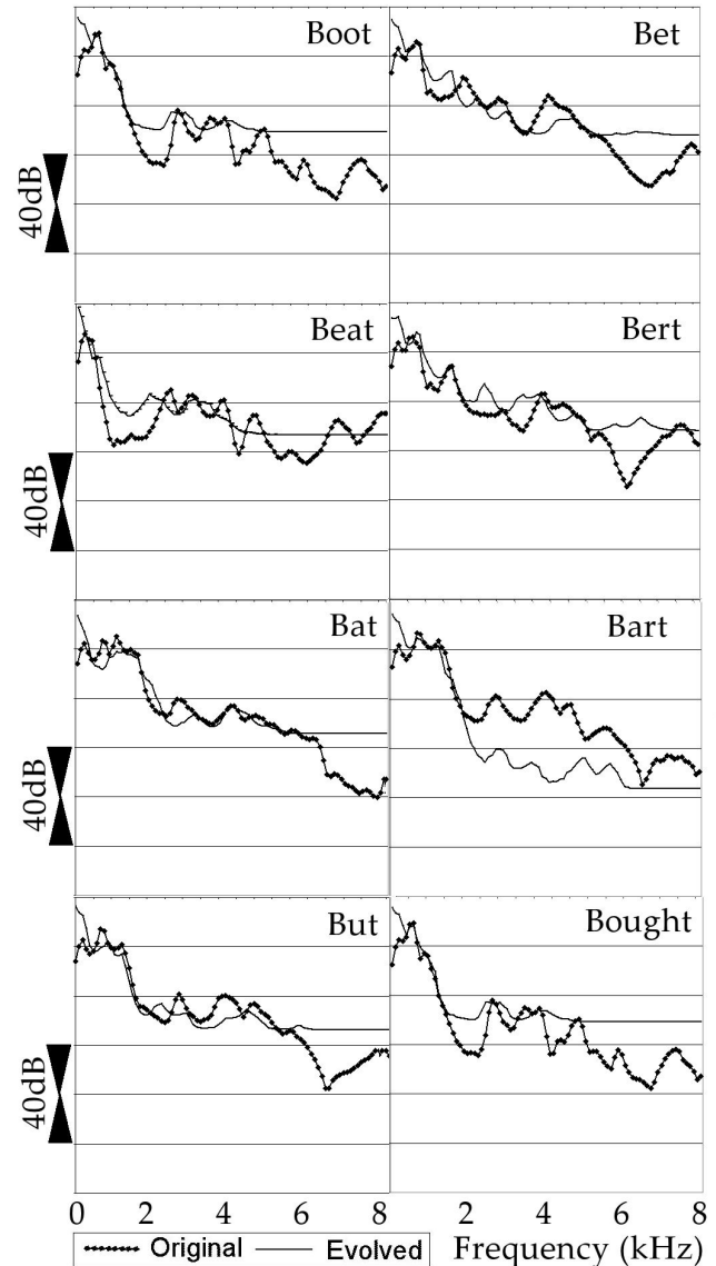
Figure 4: Long-term average spectra of the target original and evolved vowels for subject M1.
