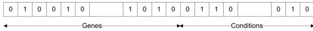
Figure 2: Encoding for the biclustering problem. In this example four genes and three conditions were chosen, so the potential bicluster has 12 elements.
