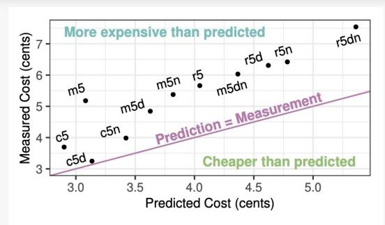
Figure 5: Prototype measurement vs. prediction on a 100 GB aggregation query
