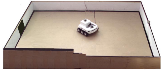
Figure 8: A mobile robot Koala equipped with a vision module gains fitness by staying near the lamp (right side) only when the light is on. The light is normally off, but it can be switched on if the robot passes near the black stripe (left side) positioned on the other side of the arena. Position of the robot is controlled by an external positioning system and passed to the computer in order to control the light and to compute the fitness.
